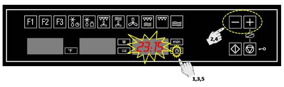
After your microwave oven is first plugged in or after a power failure, the clock display will flash to indicate that the time shown is not correct. To set the clock, proceed as follows:
